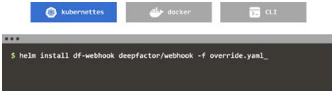
Figure 5 Installing Deepfactor's Kubernetes admission controller
