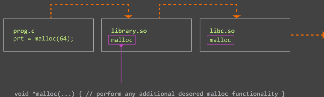
// Figure 3: Example of import table rewriting using malloc and LD_PRELOAD.
